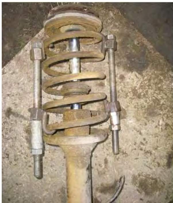
17.124.att. Amortizatora demontāža
